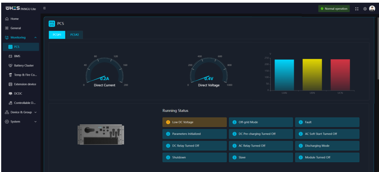
Figure 6-4 Operation Monitoring - PCS Screen
