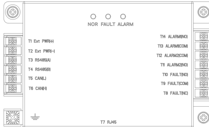
Figure 2-14 Gas Detector Module
